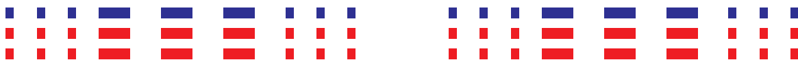
Fig. 4-2 Flashing sequence with an incorrect module or when there are no settings in the socket. A short dash corresponds to a short flash, a long dash corresponds to a long flash.
