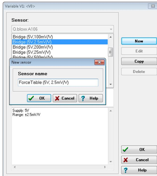
Fig. 5-5 Creating a new sensor for scaling.
