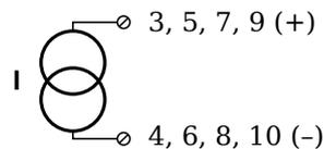
Fig. 4-28 A103, measurement of current via Q.brixx Terminal SR.
