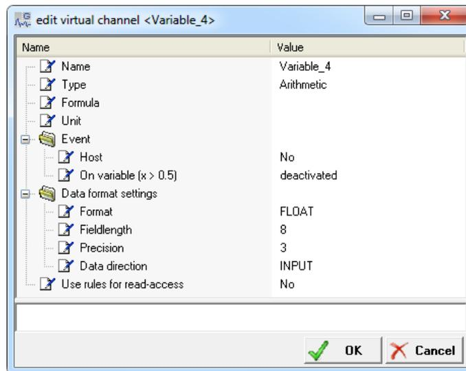
Fig. 5-14 Configuration dialog for a virtual variable.
