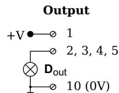
Fig. 4-81 D101, digital input and output.
