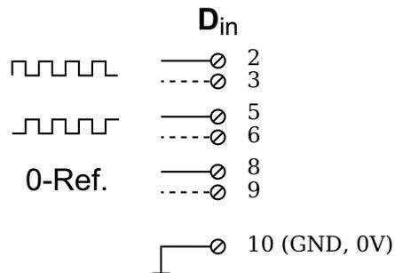
Fig. 4-90 D107, sensor with three signals (2 x 90° offset and zero reference), single-ended or differential (input broken line).
