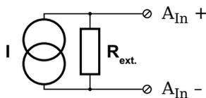
Fig. 4-77 A127, current measurement using an external shunt resistance.
