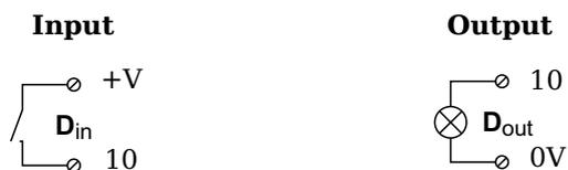
Fig. 4-17 A101, digital input and output.
