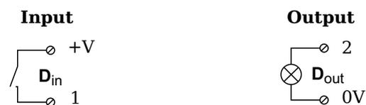
Fig. 4-29 A103, Digital Input and Output.
