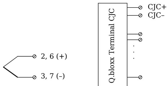
Fig. 4-48 A107, measurement with thermocouple using Q.bloxx Terminal CJC-A107.
