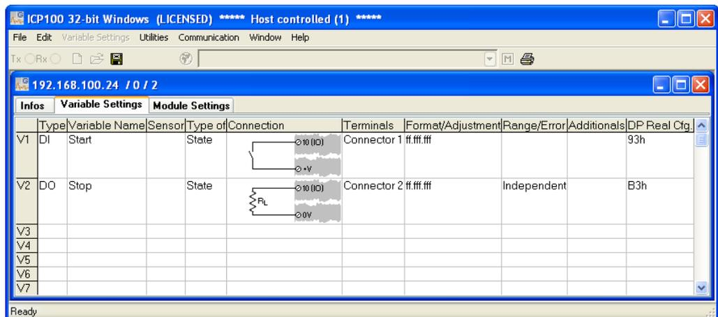
Fig. 5-8 Dialog with configuration for digital input and output.
