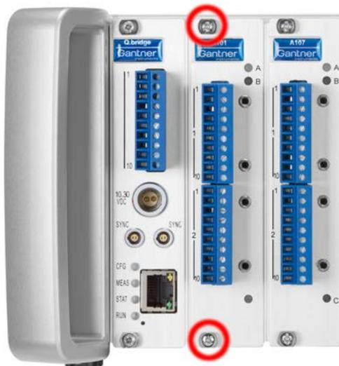
Fig. 4-92 To remove a module release the screws in the blue circles on the rear panel.
