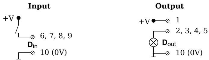
Fig. 4-58 A109, digital input and output, Plug 1.
