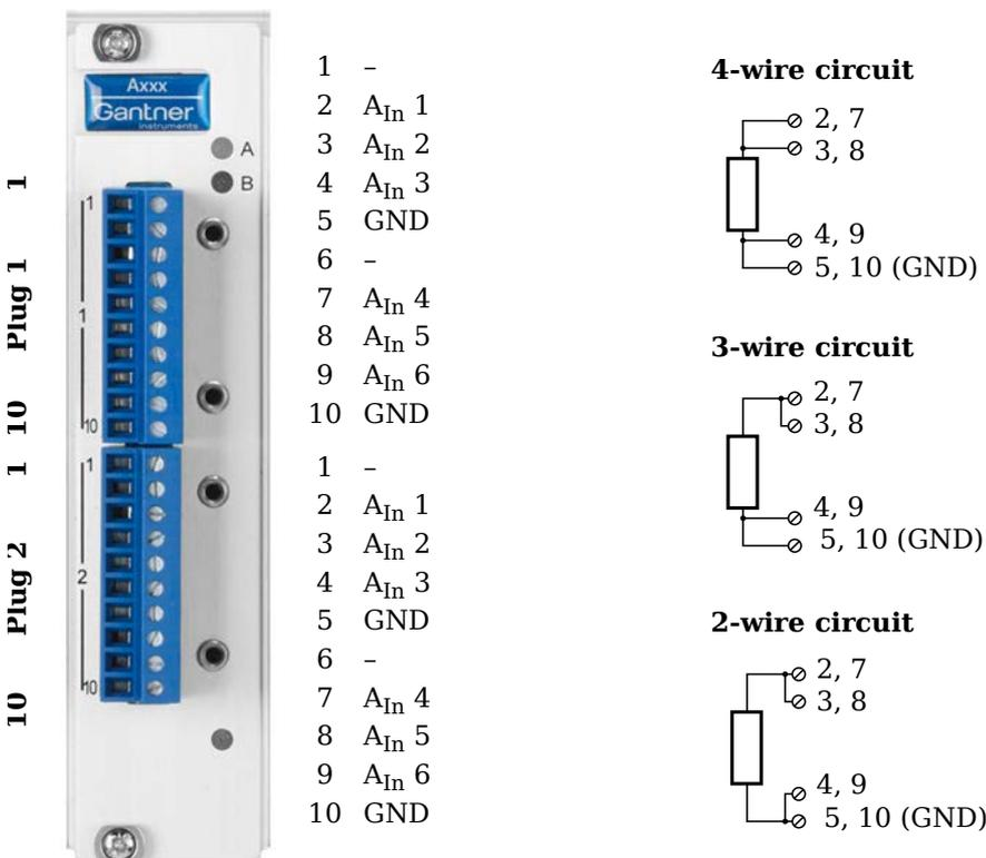
Fig. 4-33 Pin assignment for Q.brixx Module A105.
