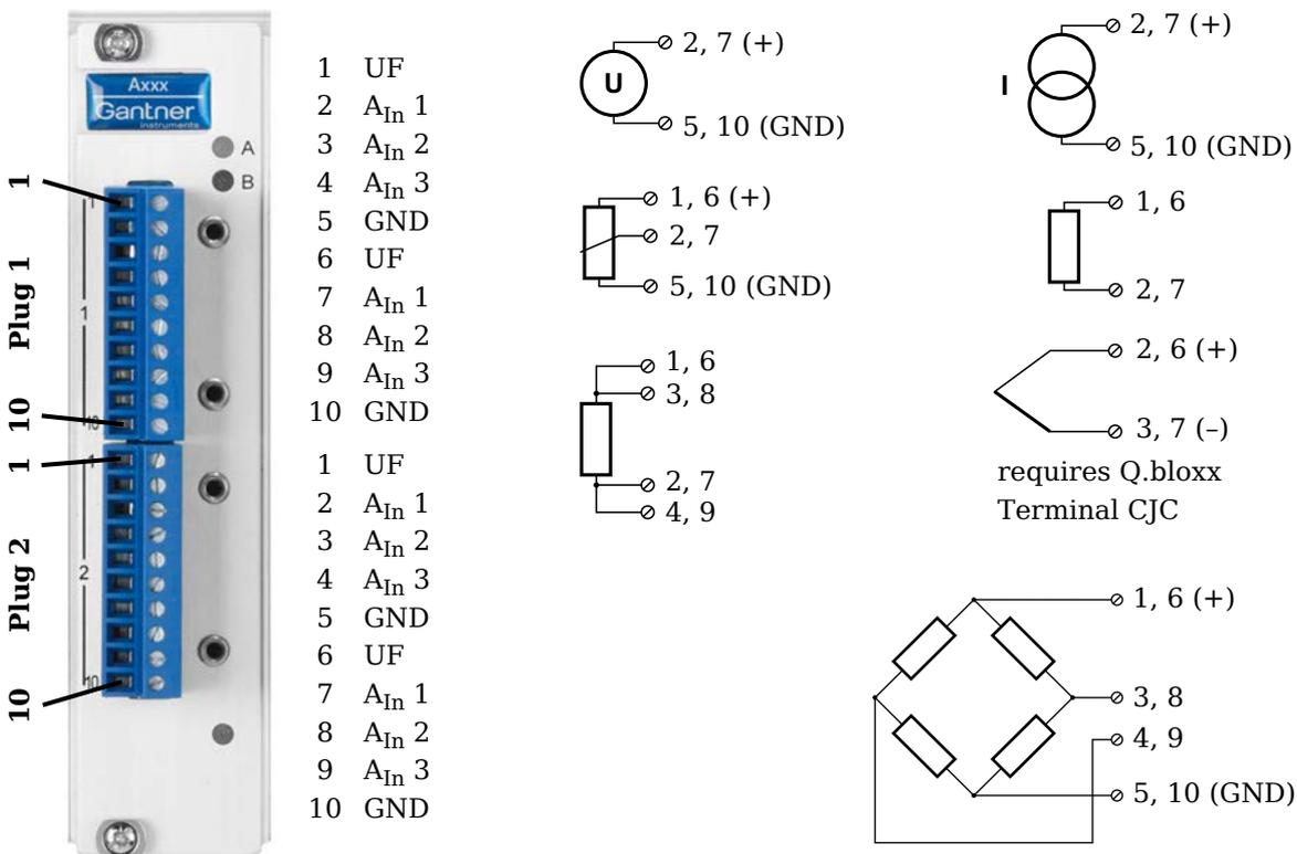
Fig. 4-42 Pin assignment for Q.brixx Module A107 (terminal version).
