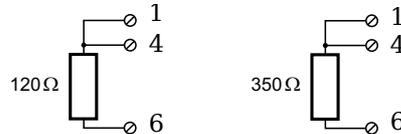
Fig. 4-22 A102, measurement with strain-gauge quarter bridge using Q.bloxx Terminal B4 on Plug 2.
