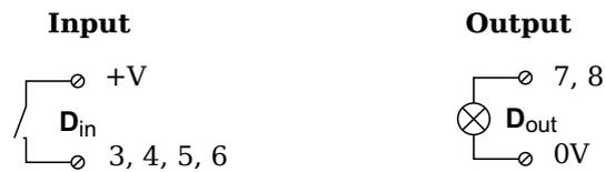
Fig. 4-25 A102, digital input and output, Plug 1.
