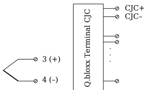
Fig. 4-13 A101, measurement with thermocouple using Q.bloxx Terminal CJC-A101.
