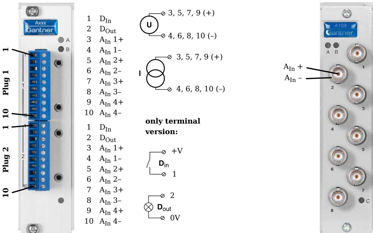
Fig. 4-53 Pin assignment for Q.brixx Module A108 (left), version with BNC sockets on the right side.
