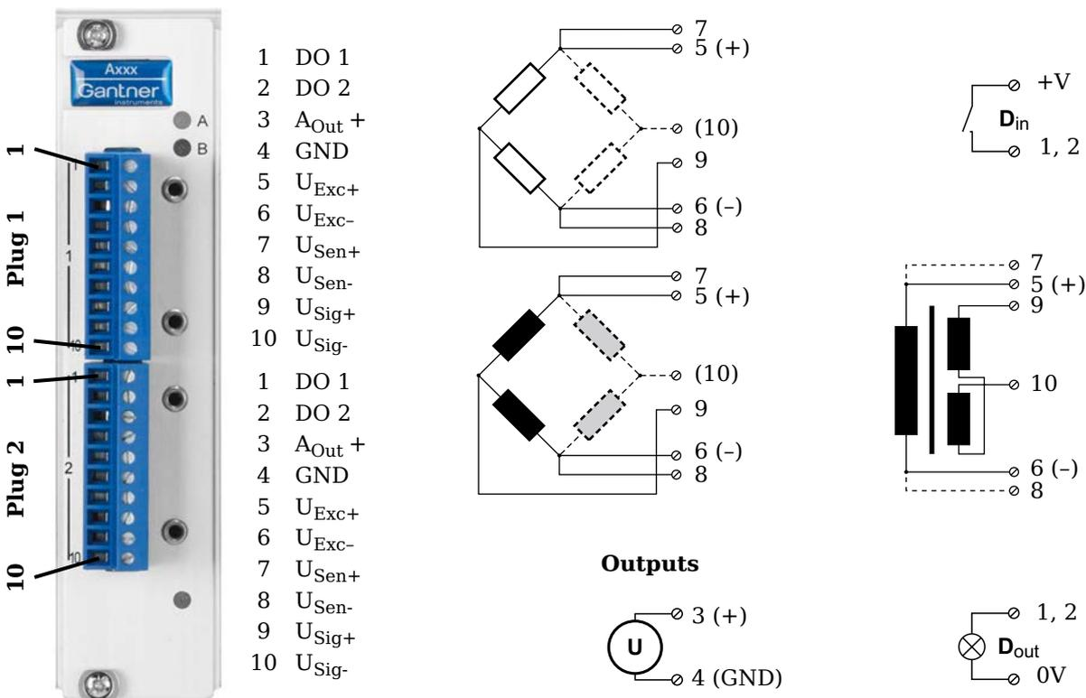
Fig. 4-35 Pin assignment for Q.brixx Module A106.
