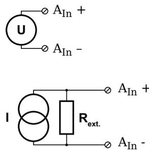
Fig. 4-75 Pin assignment for Q.brixx Module A127.
