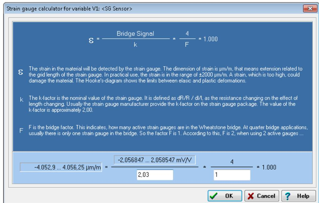
Fig. 6-7 Scaling dialog for strain gauges.
