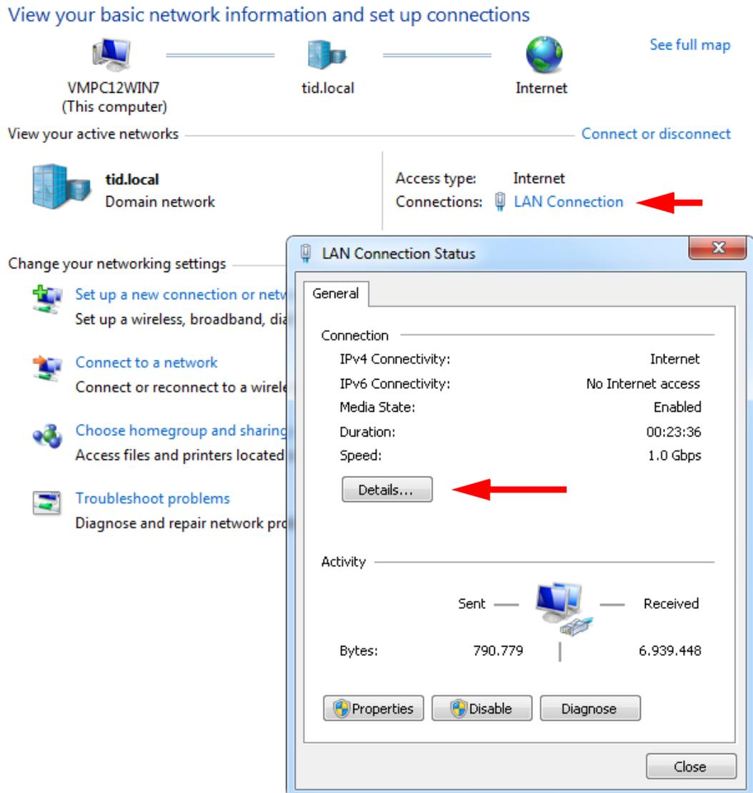
Fig. 6-1 Viewing/changing the IP address of the PC
