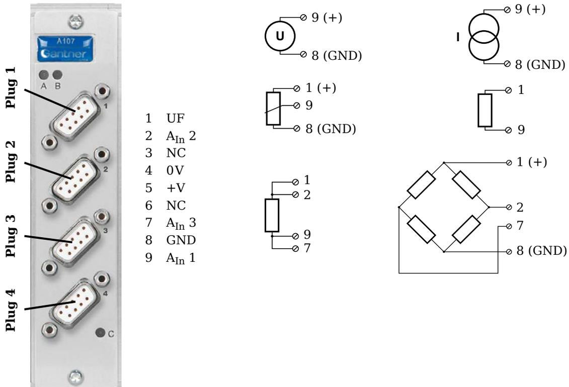
Fig. 4-43 Pin assignment for Q.brixx Module A107, version with D-sub sockets.
