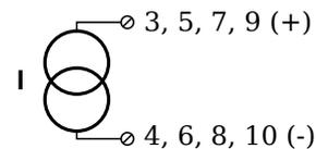
Fig. 4-57 Pin assignment for Q.brixx Module A109.
