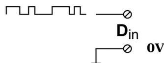
**Up/down counter or measurement of frequency and direction with static direction signal, 2 signals**
