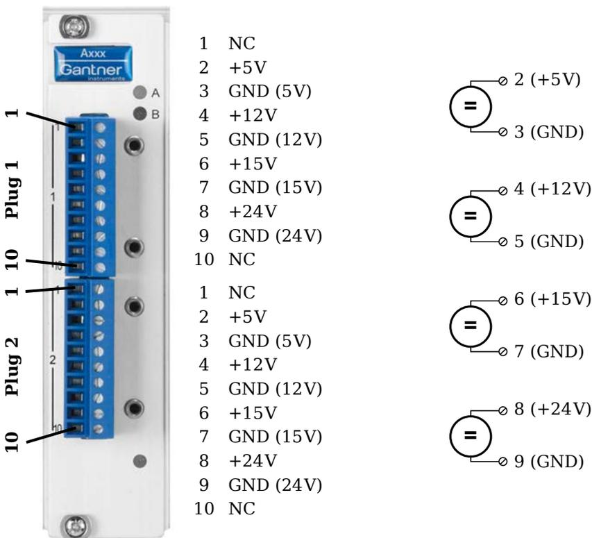
Fig. 4-91 Pin assignment for Q.brixx Module S104.
