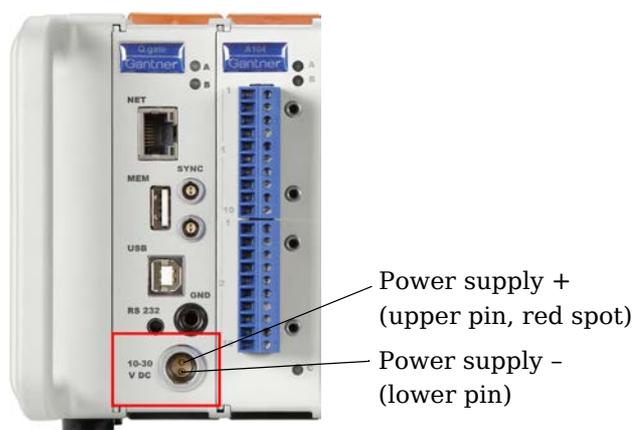
Fig. 4-1 Pin assignment on the power supply socket.
