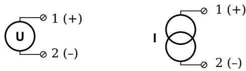
Fig. 4-24 A102, output of voltage or current, Plug 1.
