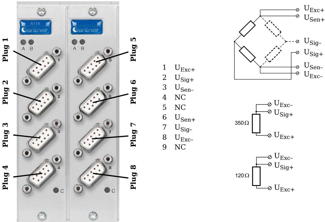
Fig. 4-63 Pin assignment for Q.brixx Module A116.
