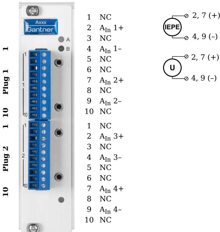
Fig. 4-60 Pin assignment for Q.brixx Module A111.
