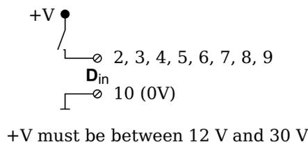
Fig. 4-82 Pin assignment for Q.brixx Module D104.
