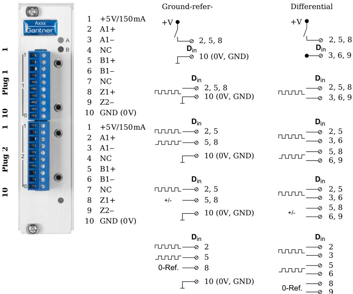
Fig. 4-86 Pin assignment and circuit variants for the Q.brixx Module D107.
