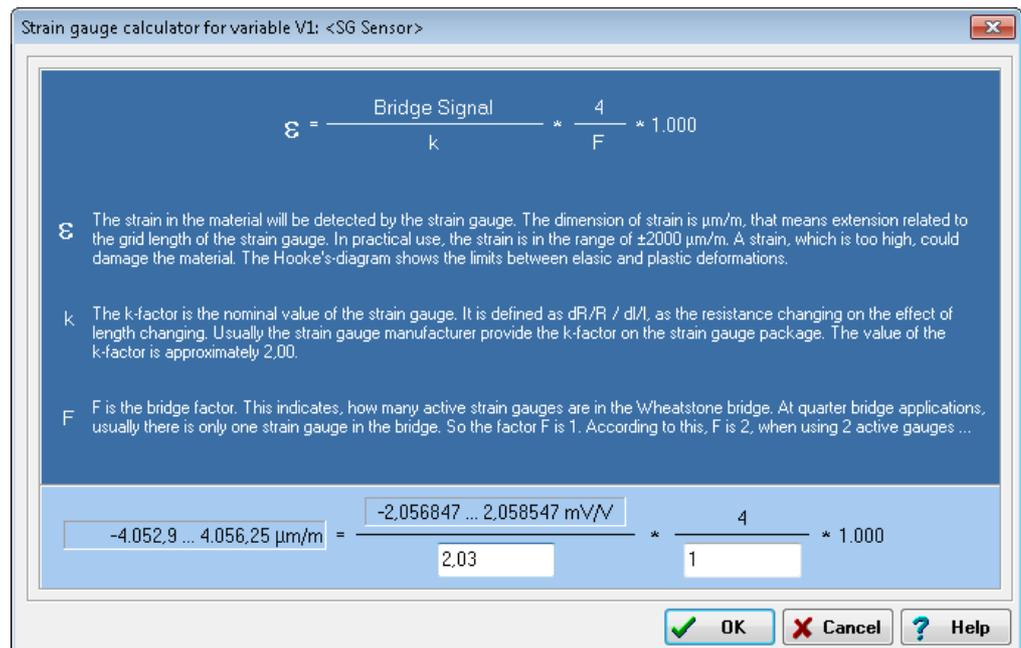
Fig. 6-7 Scaling dialog for strain gauges.
