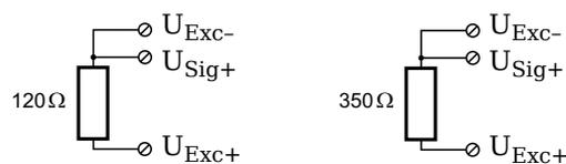
Fig. 4-65 A116, measurement with a strain-gauge quarter bridge, direct connection.
