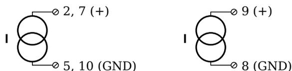
Fig. 4-45 A107, measurement of current; left: terminal version; right: D-sub sockets.
