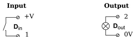
Fig. 4-29 A103, Digital Input and Output.
