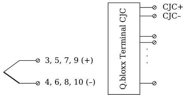
Fig. 4-32 A104, measurement with thermocouple using Q.bloxx Terminal CJC-A104.
