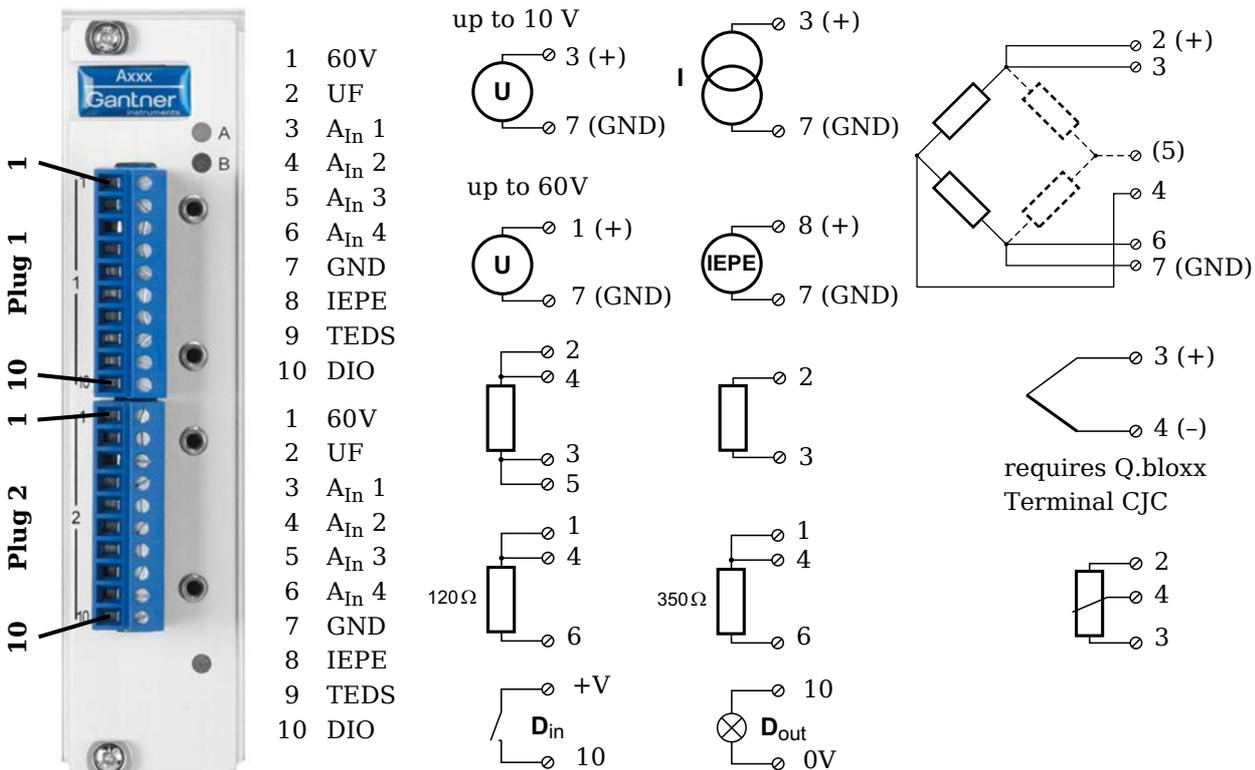
Fig. 4-8 Pin assignment for Q.brixx Module A101.
