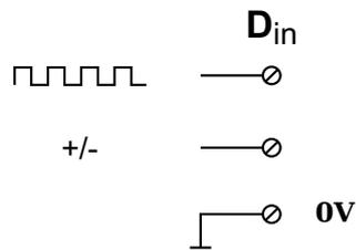
**Measurement of frequency and direction or up/down counter with 2-channel frequency signal (90° phase delay)**
