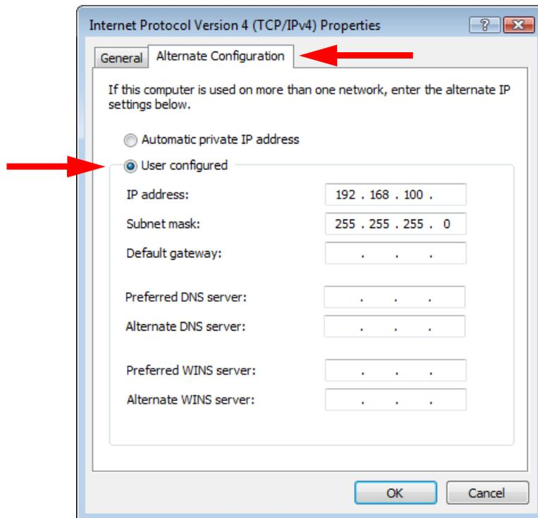
Fig. 6-3 Specifying the IP address and subnet mask for an alternative (temporary) configuration.
