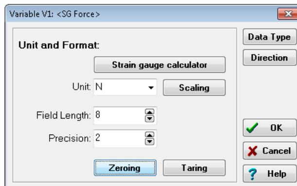
Fig. 5-3 Dialog for sensor scaling.
