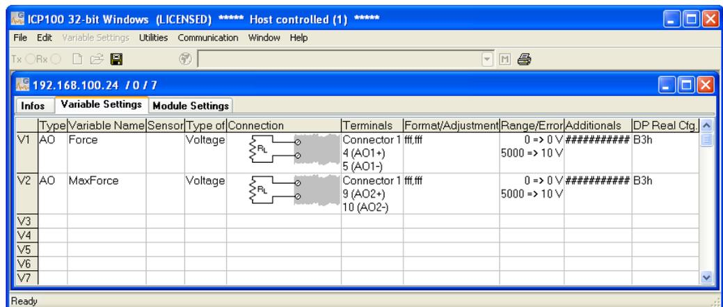
Fig. 5-9 Dialog with configuration for analog outputs.
