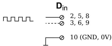
Fig. 4-87 D107, sensor with one signal, single-ended or differential (input broken line).
