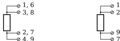
Fig. 4-47 A107, measurement of resistance and Pt100/1000 probes; left: terminal version; right: D-sub sockets.
