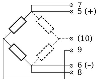
Fig. 4-36 A106, measurement with full and half bridges.
