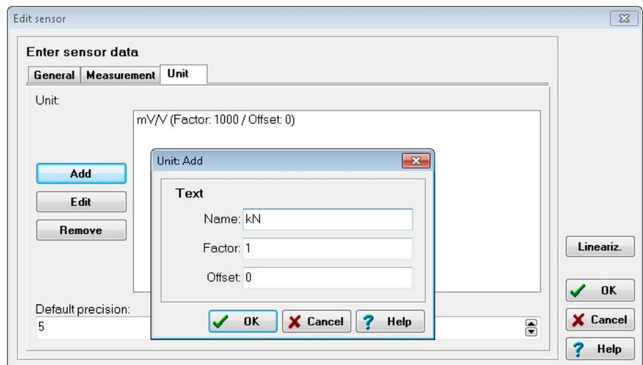
Fig. 5-6 Defining the unit for sensor scaling.
