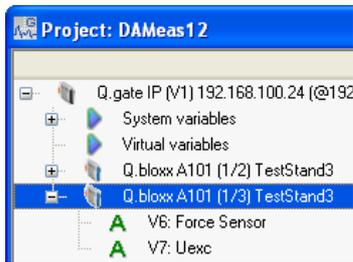
In order to set parameters you should be connected to the module and have called the configuration program (ICP 100 which is started automatically by test.commander): Mark a module and select **Configuration** from the context menu or double click on a module or module signal (variable) to start the configuration program. Then carry out all the module settings in the window of this program.
