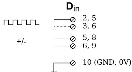
Fig. 4-88 D107, sensor with two signals (counting direction), single-ended or differential (input broken line).
