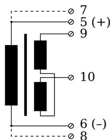
Fig. 4-39 A106, measurement with LVDTs and RVDTs.
