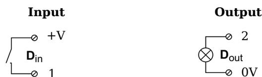
Fig. 4-56 A108, digital input and output.
