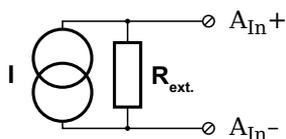
Fig. 4-71 A123, current measurement using an external shunt resistance.
