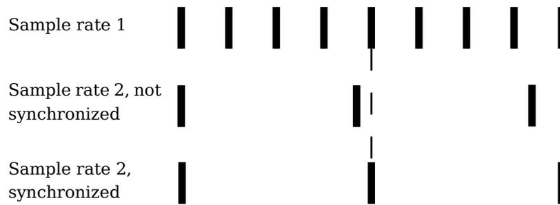
Fig. 5-12 Data transmission at a synchronous sampling frequency.
