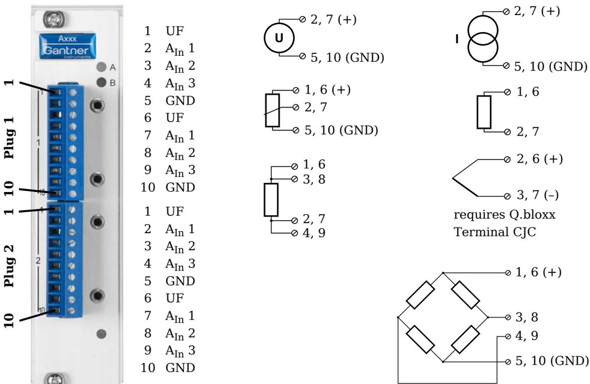
Fig. 4-42 Pin assignment for Q.brixx Module A107 (terminal version).
