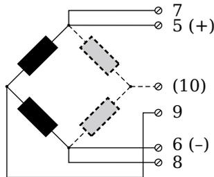
Fig. 4-38 A106, measurement with inductive full and half bridges.
