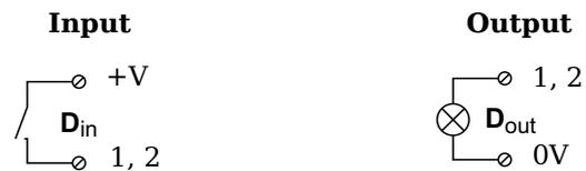
Fig. 4-41 A106, Digital Input and Output.
