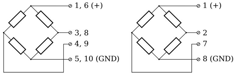
Fig. 4-49 A107, measurement with full bridge; left: terminal version; right: D-sub sockets.
