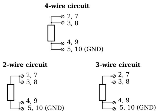
Fig. 4-34 A105, measurement of resistance and Pt100/1000 probes.
