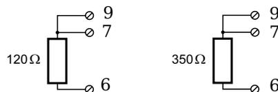
Fig. 4-37 A106, measurement with strain-gauge quarter bridge using Q.bloxx Terminal B4.
