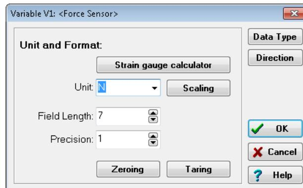
Fig. 6-5 Setup dialog for scaling.
