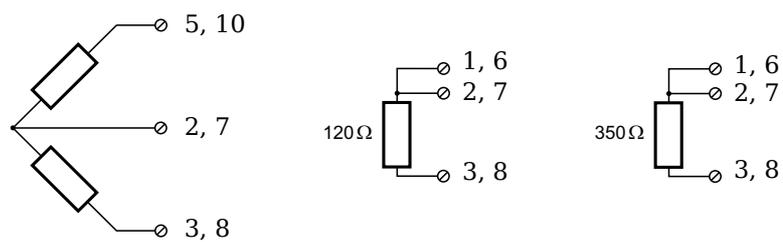
Fig. 4-51 A107, measurement with strain-gauge half bridge and quarter bridge using Q.bloxx Terminal B4 (terminal version).
