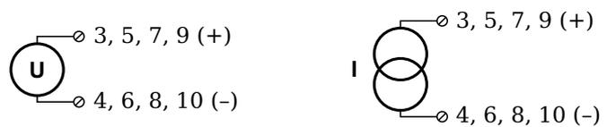
Fig. 4-59 A109, output of voltage or current, Plug 2.
