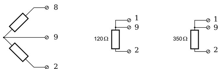
Fig. 4-52 A107, measurement with strain-gauge half bridge and quarter bridge through adapter plug on the version with D-sub sockets.
