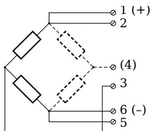
Fig. 4-21 A102, measurement with full and half bridges, Plug 2.
