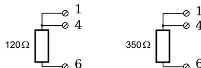
Fig. 4-15 A101, measurement with strain-gauge quarter bridge using Q.bloxx Terminal B4.
