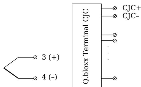
Fig. 4-13 A101, measurement with thermocouple using Q.bloxx Terminal CJC-A101.
