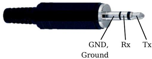
Fig. 4-2 Pin assignment for RS-232 on the jack plug.
