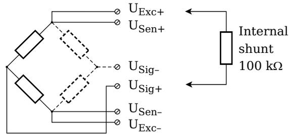
Fig. 4-64 A116, measurement with full and half bridges;  $U_{SIG}$  = signal voltage (output signal),  $U_{SEN}$  = sense lead,  $U_{EXC}$  = excitation voltage
