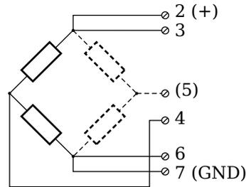
Fig. 4-14 A101, measurement with full and half bridges.
