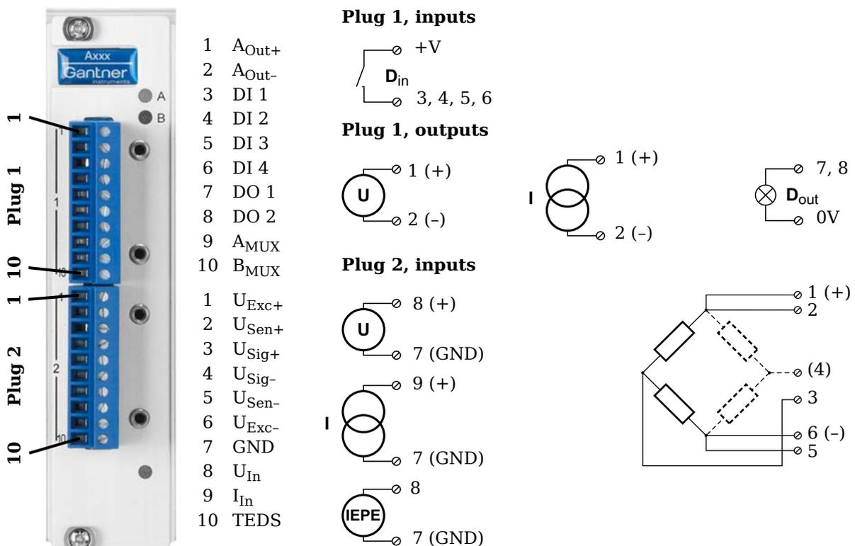
Fig. 4-18 Pin assignment for Q.brixx Module A102.
