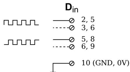
Fig. 4-89 D107, sensor with two signals (90° offset), single-ended or differential (input broken line).
