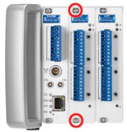
Abb. 4-72 To remove a module release the screws in the red circles.
