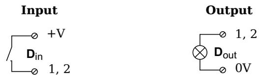
Abb. 4-33 A106, Digital Input and Output.
