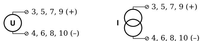
Abb. 4-51 A109, output of voltage or current, Plug 2
