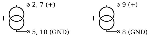
Abb. 4-37 A107, measurement of current; left: terminal version; right: D-sub sockets.
