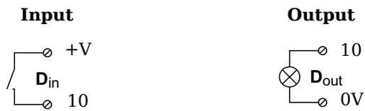
Abb. 4-15 A101, digital input and output.
