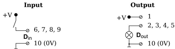
Abb. 4-50 A109, digital input and output, Plug 1.
