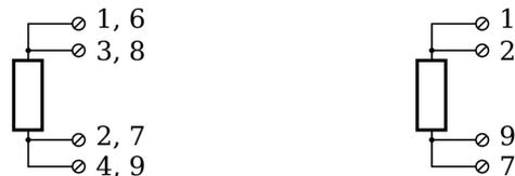
Abb. 4-39 A107, measurement of resistance and Pt100/1000 probes; left: terminal version; right: D-sub sockets.
