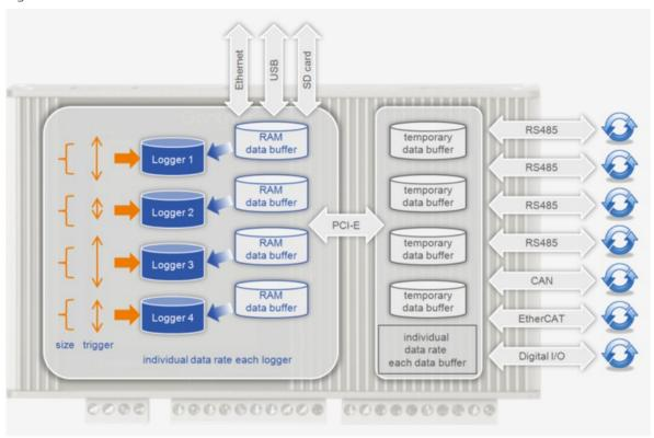
According to the configuration of up to 20 loggers occurs the logging of the buffer data at a selectable medium (intern. Flash, USB, SD-Card) with selectable logging rates, storage duration, start and stop trigger (auto start, condition, touch) with or without pre- and post-trigger.
