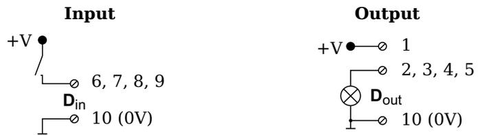
Fig. 5-52 A109, digital input and output, Plug 1.
