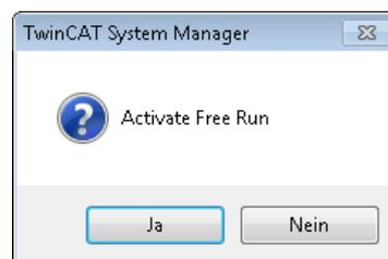
Fig. 6-24 Activating the “Free Run” operating mode.
