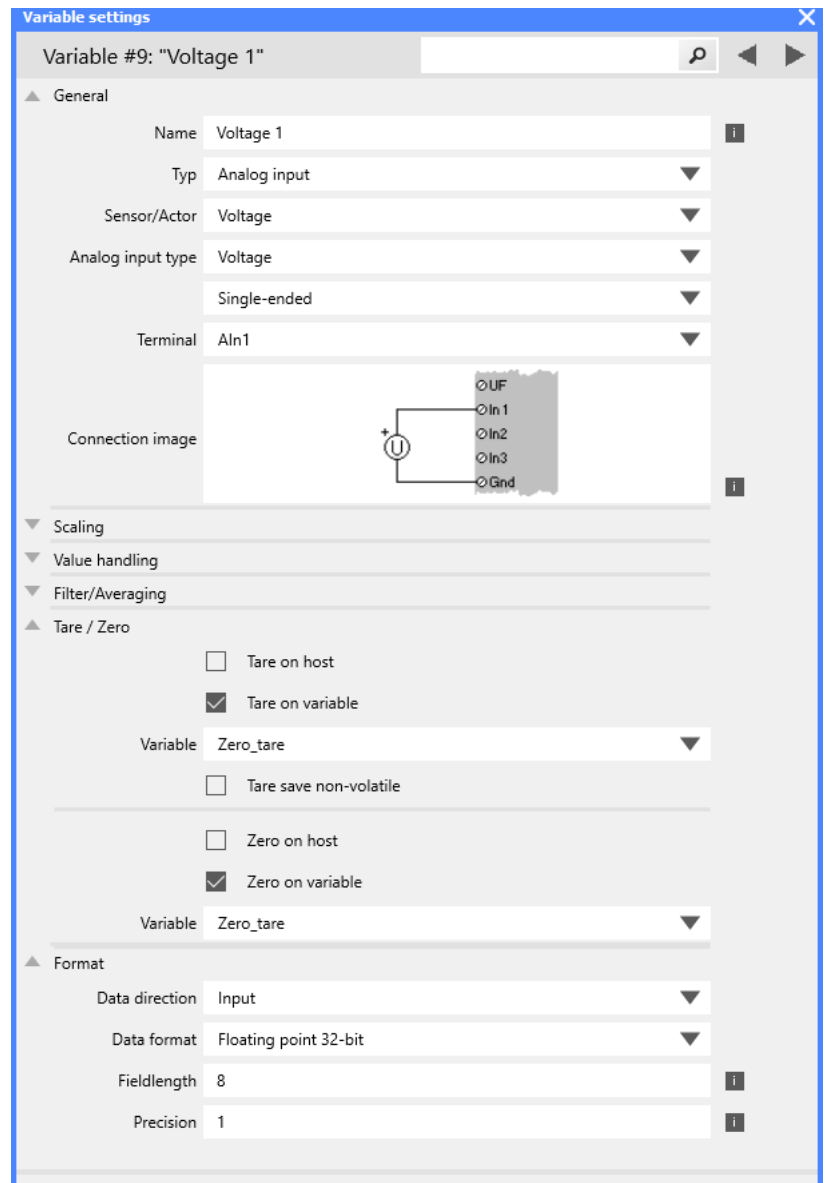
Fig. 8-3 Define the desired conditions for Zero and/or Tare
