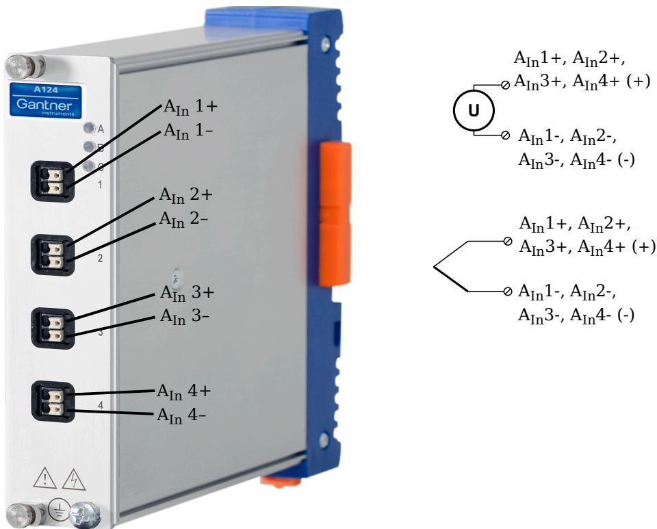
Fig. 5-80 Pin assignments for Q.series XL A124
