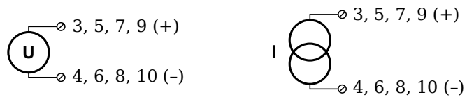
Fig. 5-56 A109, terminal wiring configurations for analog output of voltage or current, available via Terminal 2 only
