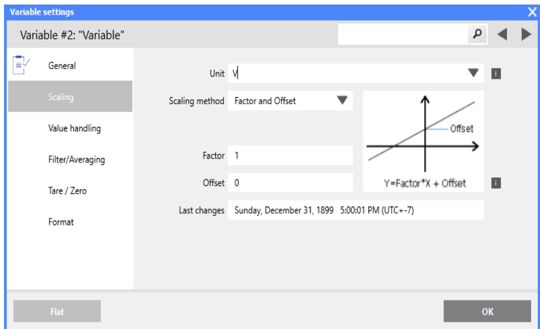
Fig. 11-4 Scaling options for voltage using Factor and Offset
