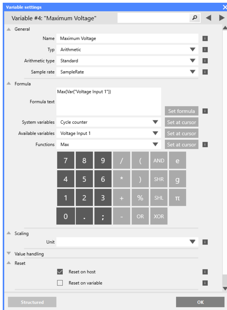
Fig. 7-14 Defining an arithmetic virtual variable with reset on host
