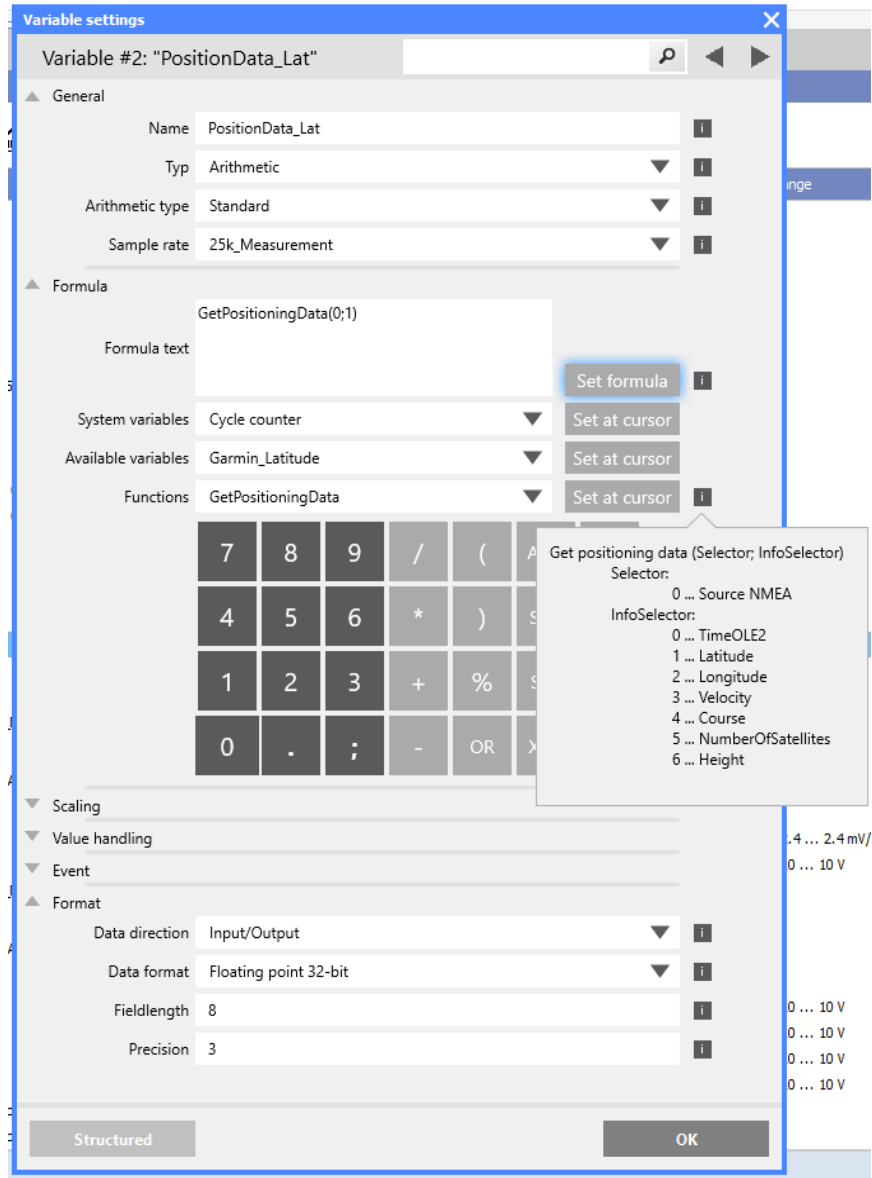
Fig. 6-6 Output of the latitude (Parameter = 1) via variable type Arithmetic; the NMEA receiver is connected to USB1 (Parameter = 0; Source NMEA)
