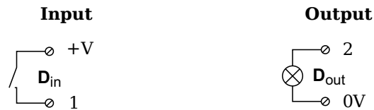
Fig. 5-53 A108, terminal wiring configurations for digital input and output, available for terminal versions only
