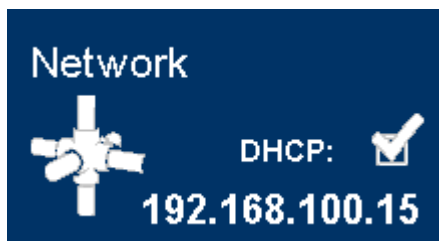
Fig. 6-1 Network tile with view of the IP address in the HMI
