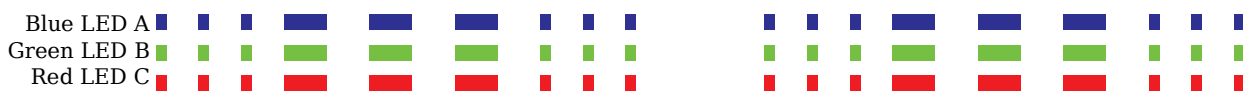
Fig. 4-10 Flashing sequence indicating an incorrect module type or there are no configurations stored in the socket
