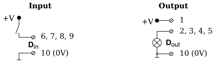
Fig. 5-55 A109, terminal wiring configurations for digital input and output, available via Terminal 1 only
