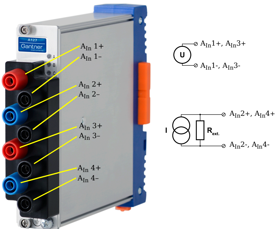
Fig. 5-83 Connection assignments for the Q.series XL A127
