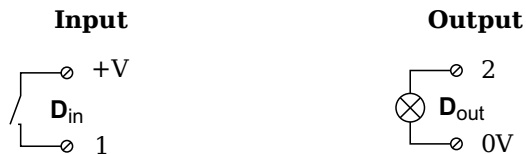
Fig. 5-58 A108, terminal wiring configurations for digital input and output, available for terminal versions only
