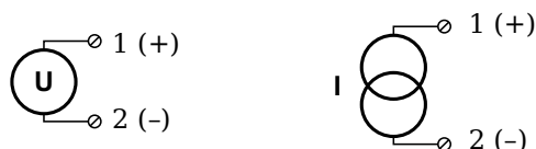
Fig. 5-29 A102, terminal wiring configuration for analog output of voltage or current, available via Terminal 1 only
