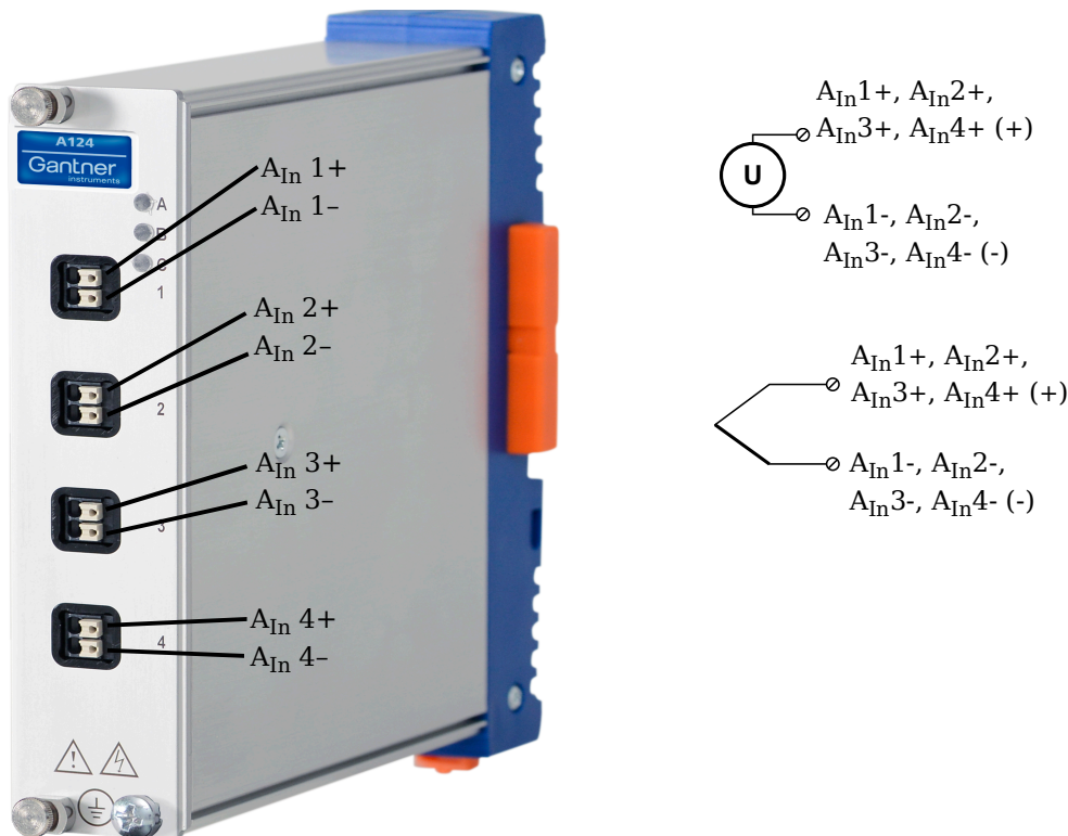
Fig. 5-84 Pin assignments for Q.series XE A124
