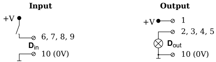
Fig. 5-60 A109, terminal wiring configurations for digital input and output, available via Terminal 1 only
