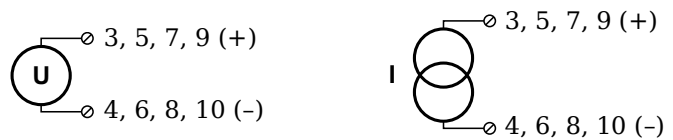
Fig. 5-61 A109, terminal wiring configurations for analog output of voltage or current, available via Terminal 2 only
