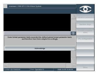
Tolerances can be set on a global level by the administrator. Thus, the user can only operate within these frames when making changes. This increases production security.
