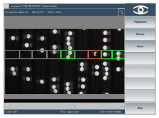
Evaluation on a vibratory feeder. The separating of the products that are randomly distributed on the lanes is undertaken by the software. Afterwards, product inspection takes place.
