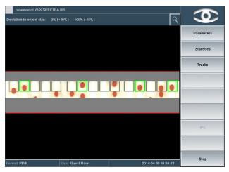
Evaluation of soft gel bulk. Due to irregular arrangements, the separation of the products is crucial.
