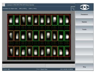
Evaluation on a slat counter. The upright products are inspected and signals processed. The screenshot shows cross-contamination with smaller objects.
