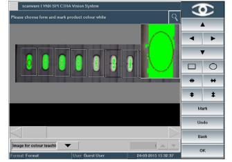
Camera-specific colour tolerances can have a negative impact on evaluation. The software feature "Colours per Camera" determines that colour values are set for each camera individually during teach-in. This eliminates camera-based irregularities and facilitates precise evaluation. The user, however, teaches on one image.
