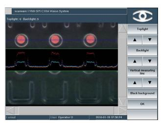
For Japan Quality Product Inspection, even the slightest degree of reflections can be problematic. The measuring line used by scanware enables the setting of safe, reproducible settings for the W-LED illumination. The line can be used vertically, for example if multiple camera images appear one underneath the other.
