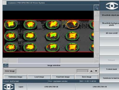
Evaluation of a blister filled with powder pellets. The pocket with insufficient powder is detected despite the irregular shapes the powder takes in the pocket.
