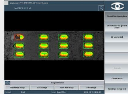
Evaluation of pockets filled to the rim. Missing powder is detected by the system.
