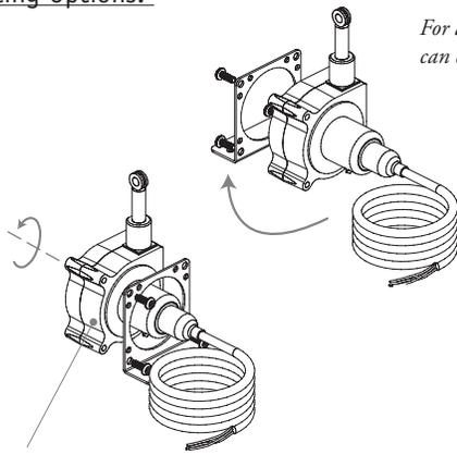
For added flexibility, mounting bracket can easily be switched to the opposite side.
