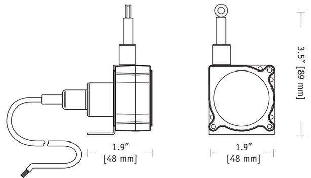
The SP2 String Pot from Celesco is a compact, economical and water resistant device that utilizes a flexible cable, a spring-loaded spool and a potentiometer to detect and measure linear position.
