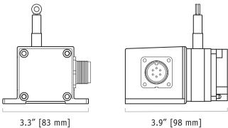
The PT1DC can operate from an unregulated 14.5 to 40 VDC power supply while providing an output signal that is proportional to the linear movement of it's measuring cable. The PT1DC has a maximum measurement range up to 50" and has 4 output signal options to choose from: 0...10, 0...5, -10...+10 and -5...+5 Vdc.
