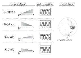
The output signal direction can be reversed at any time by simply changing the dip-switch settings found on the internal signal board. After the settings have been changed, adjustment of the Zero and Span trimpots will be required to precisely match signal values to the beginning and end points of the stroke.
