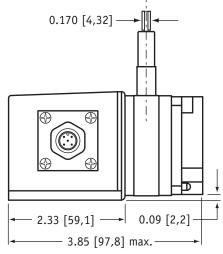
\* tolerance = +.005 -.001 [+.13 -.03] \*\* tolerance = +.005 -.005 [+.13 -.13]
