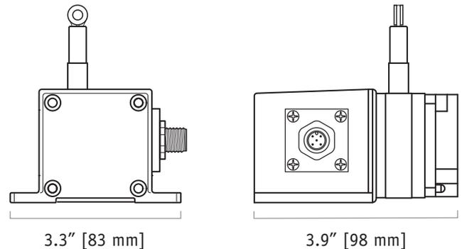
The PT1DN communicates to your PLC over DeviceNET® and provides a precision position feedback signal for full-scale measurement ranges from 2 to 50 inches. Because the PT1DN uses a potentiometer as its sensing element, the position signal is “absolute” and does not have to be reset to a “home” position upon startup.
