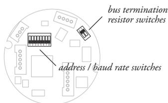
to gain access to the controller board, remove four Allen-Head Screws and remove rear cover.
