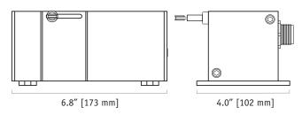
The PT5AV is a combination position and velocity transducer. A precision plastic-hybrid potentiometer provides accurate position feedback while a self-generating DC tachometer provides a velocity signal that is proportional to the speed of the traveling measuring cable.
