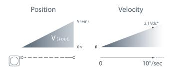
\*velocity output rate =  $354 \text{ mV} \pm 4\%$  @ 100 inches per min.
