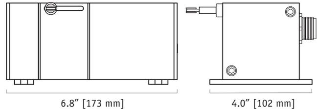
The PT5DC cable-extension transducer uses a unique thermoplastic cable that has virtually an infinite fatigue life. This cable, known as V62, has properties that are superior for high cycle and rugged applications.
