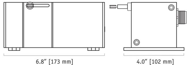
The PT5DN, using a high cycle plastic-hybrid potentiometer, communicates via DeviceNET protocol with programmable controllers in factories and harsh environments requiring linear position measurements in ranges up to 250".
