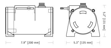
The PT9101 is a work-horse for demanding long-range applications requiring a linear position measurements in ranges up to 1700 inches. Available with either a 500, 1K, 5K, or 10K ohm potentiometer, the PT9101 operates with any basic panel meter or programmable controller.
