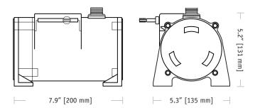
The PT9232 delivers position feedback via RS232 serial communication to your data acquisition or controller system. The PT9232 sends a raw 16-bit count from 0000H to FFFFH. Additionally this device can be set to continuously send data or send data only when polled.
