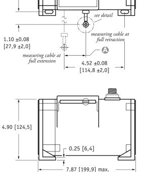
DIMENSIONS ARE IN INCHES [MM] tolerances are 0.03 IN. [0.5 MM] unless otherwise noted.
