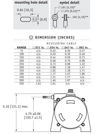
\* tolerance = +.005 -.001 [+.13 -.03] \*\* tolerance = +.005 -.005 [+.13 -.13]
