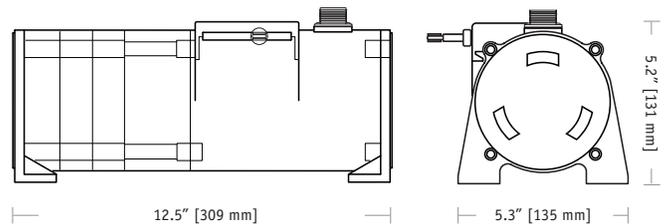
The PT9301 is a combination position and velocity transducer for demanding long-range applications requiring a linear position measurements in ranges up to 1700". A precision plastic-hybrid potentiometer provides accurate position feedback while a self-generating DC tachometer provides a velocity signal that is proportional to the speed of the traveling stainless-steel measuring cable.
