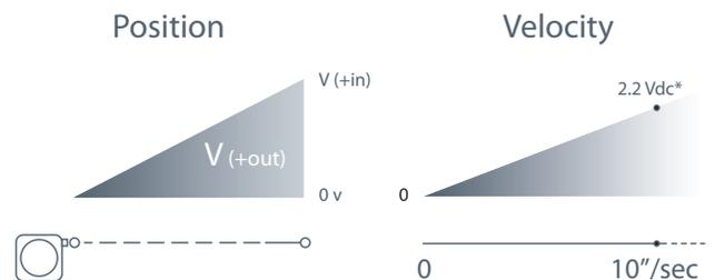
\*velocity output rate = 361 mV  $\pm 3\%$  @ 100 inches per min.
