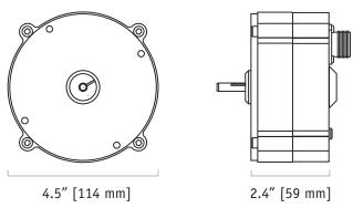
Celesco's model RT9DN communicates rotational position feedback via DeviceNET® to your programmable controller. The heart of this sensor is a precision plastic-hybrid position potentiometer which provides a "absolute" position and does not ever have to be reset to a "home" position after a power loss or planned shutdown.
