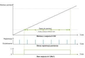
Example of trigger measurement in "1 status" mode.
