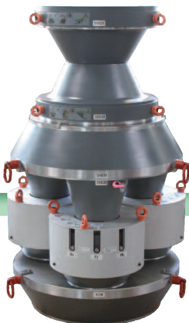
Modern force multiplication: Build-up 30MN
