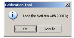
9) Load onto the scale the corresponding weight and confirm the "**OK**"; the following appears:
