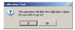
By confirming the window, a calibration point equal to the scale capacity will be entered (marked in the screenshot):
