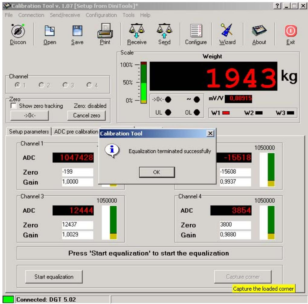
After the acquisition, the message "Equalization terminated successfully" appears, press on OK.
