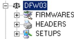
With this menu it is possible to transmit to the indicator a print header of up to 4 lines of 24 characters each.
