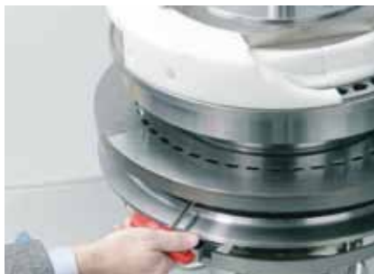
Undo chucking wedge
